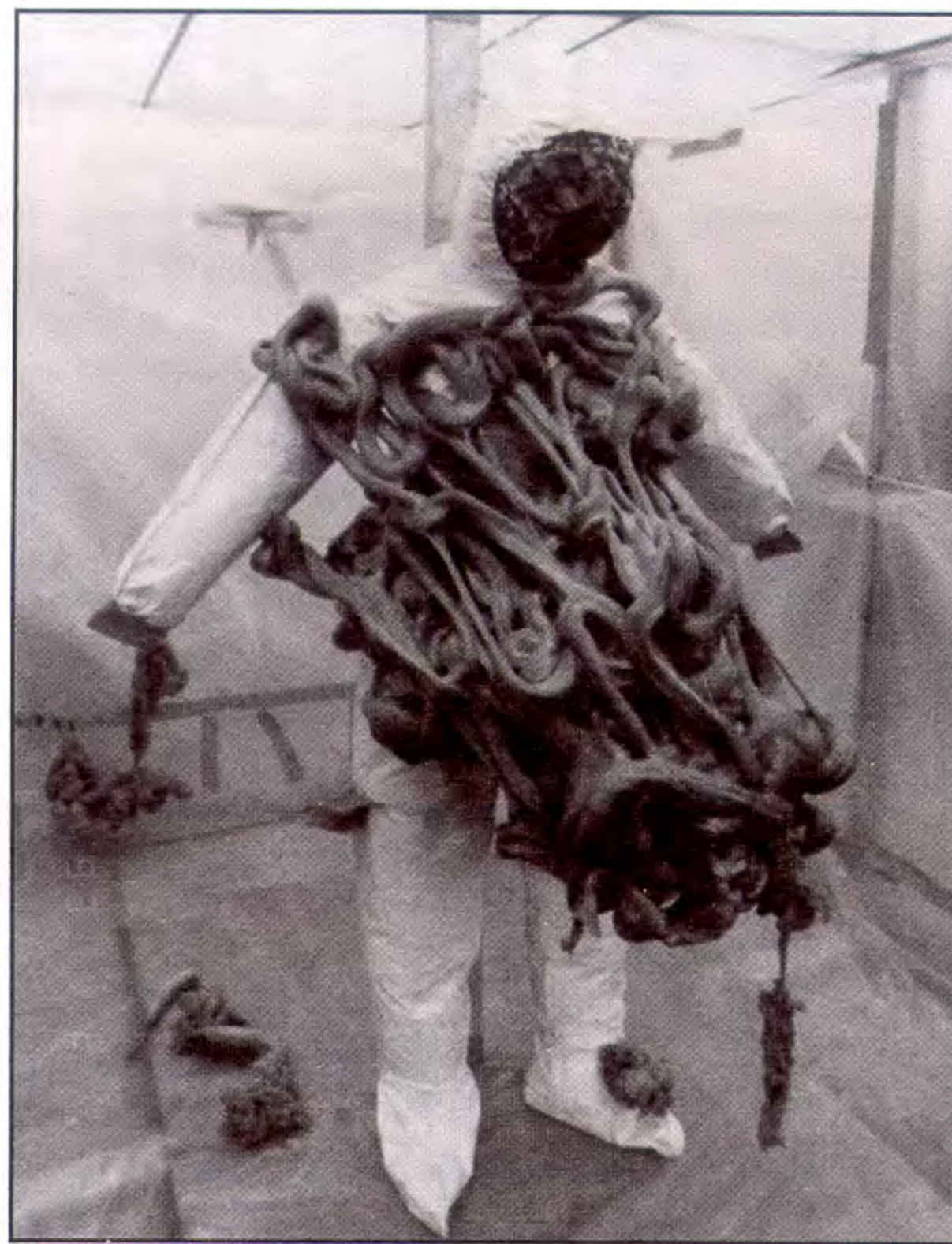
(Far left): Sticky foam is sprayed from a pressurized shoulder-slung "gun," then turns into a glue that sticks on contact (left). Experts believe the foam can disable armed individuals safely.
