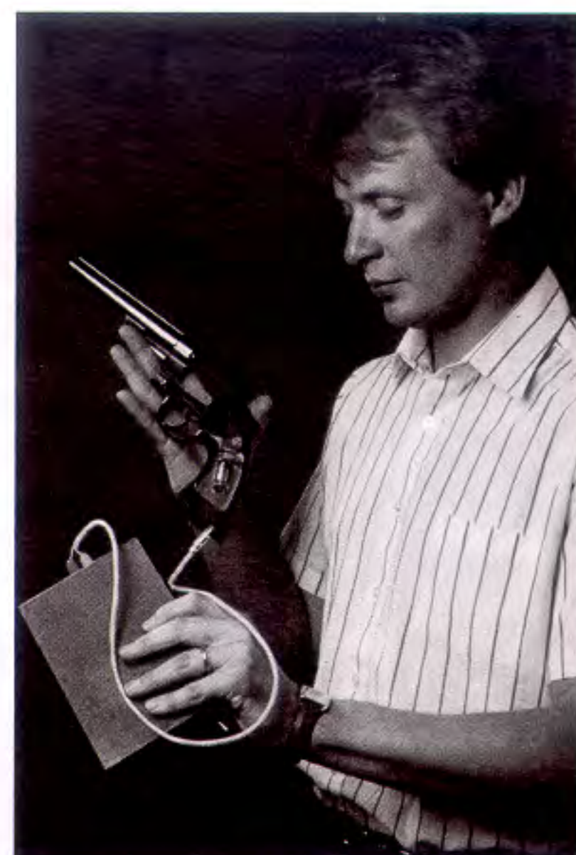
The "smart gun" (above) has sensors that would allow only the authorized user to fire it.
